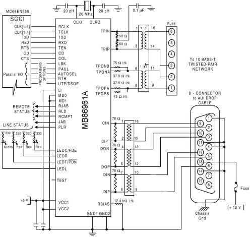
Figure 1: Interface Between the MB86961A and the MC68EN360
